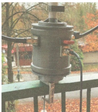
Fig. 3 ML A- S (RT/R), balcony installation, control cabinet detail. The jumper is used in all MLA- S to switch the band segment. Here the red jumper switches the antenna to the 60 m band.
